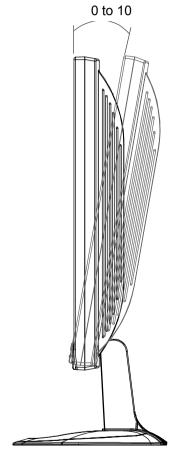
Figure 1-3: Tilting the Monitor
